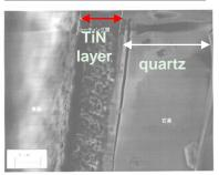
TiN coating having 2-3 mm thickness was coated on the quartz surface.
