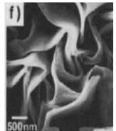
The intensity of SERS spectrum of "wrinkled Overview nanoporous metal foil" is about 60 times higher than that of nanoporous metal foil
