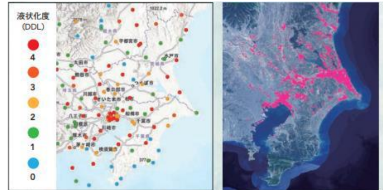
Comparison of the AI evaluation result based on seismic movement observed with K-net and KIK-net of National Research Institute
