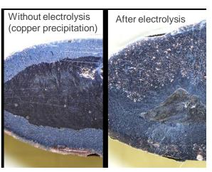
Transfer of Cu in molten iron due to electrolysis
