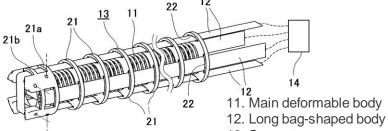
13. Support mean14. Fluid supply / discharge mean
