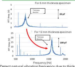
Detect natural vibration frequency due to thickness
